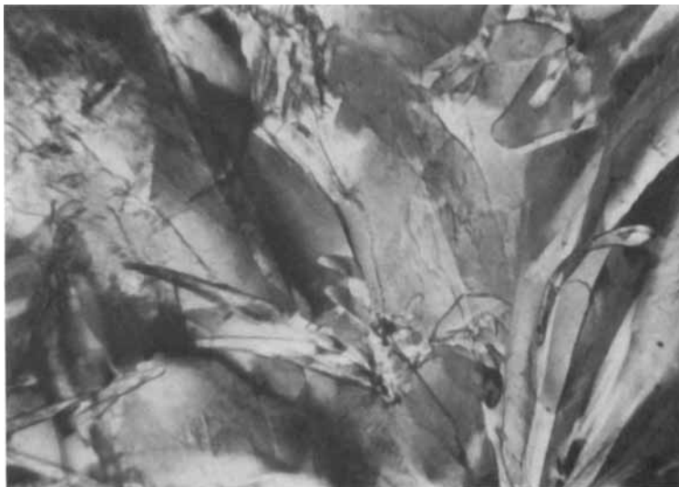
FIGURE 7a Photomicrograph Of Compound 5 on First Heating At 136.5^{\circ}\text{C} in Different Region (300X Magnification). (See Color Plate IV).
